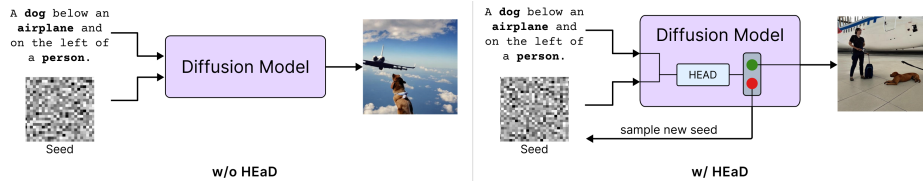
Fig. 1: Overview of the HEaD pipeline: during the generation process, HEaD assesses whether all designated objects will be accurately represented in the final image, determining if the generation process should continue or be restarted with a different seed.
